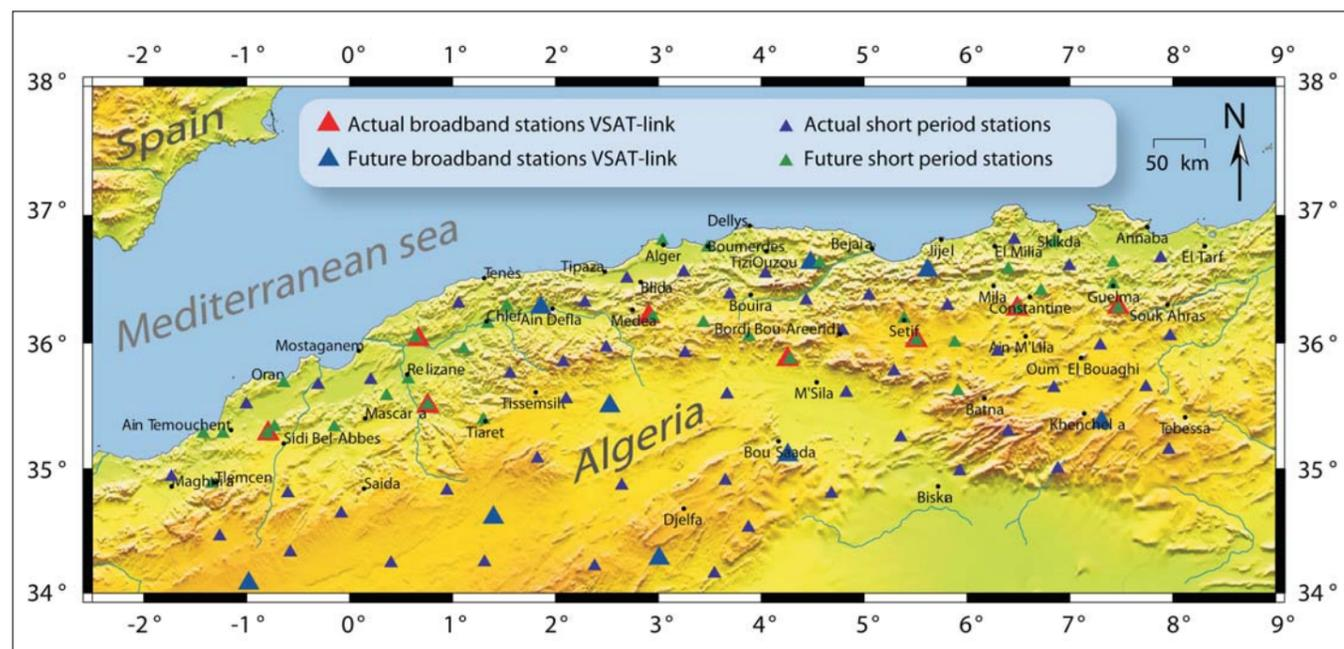
Each subnetwork is composed by a regional station with a three components sensor and some uni-component stations (SS1 short period seismometer), installed in the mountains of the Tellian chain. These later transmit their signal to the regional stations by radio-link mode.
