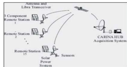
Seismological data Center near Gharyan city where the seismic data are received from all remote stations in a real-time. The seismic data which were detected at the remote stations are then transferred to the Central Hub (Seismological Data Center in Gharyan) via satellite (figure 3b and 4).
